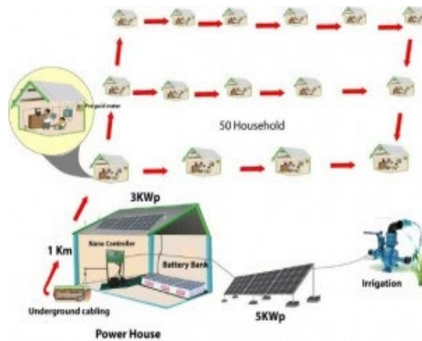
Figure 5. Pilot Nano Grid Technology. [Source: Solaric]
