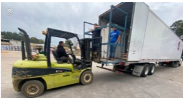
Figure 2: Current method for unloading doors.
