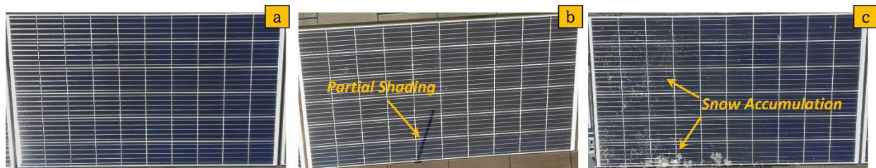
Figure 3: Samples of the Processed Images for (a) Healthy class (NO_FAULT); (b) Partial shading class (SHADING); and (c) Snow accumulation class (SNOW).
