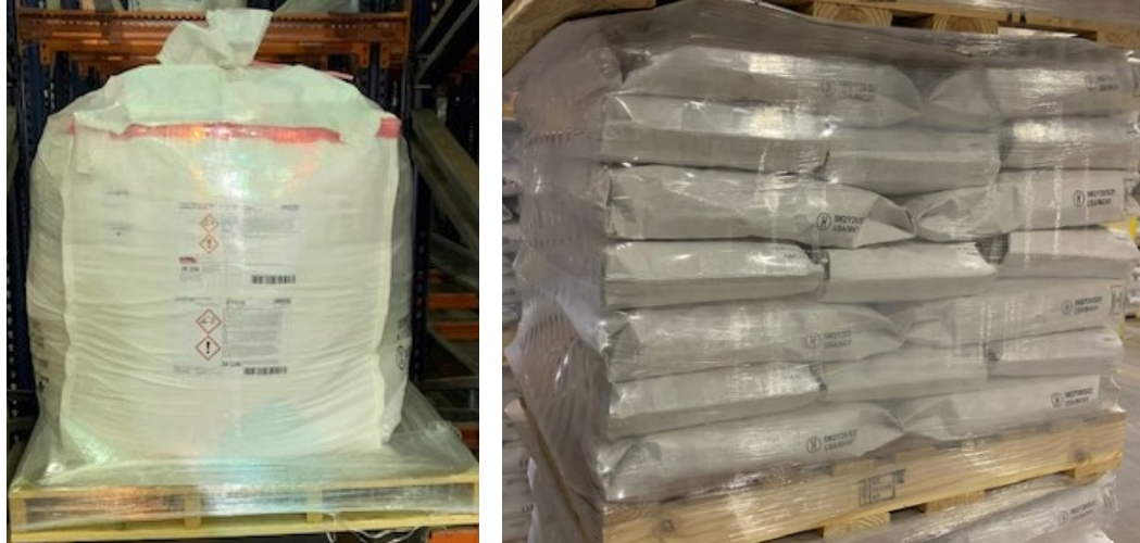
Figure 2. Examples of Package Types: One Ton Super Sack and Stacked Pallet of Twenty-Five-kilogram Poly-lined Paper Bags.
