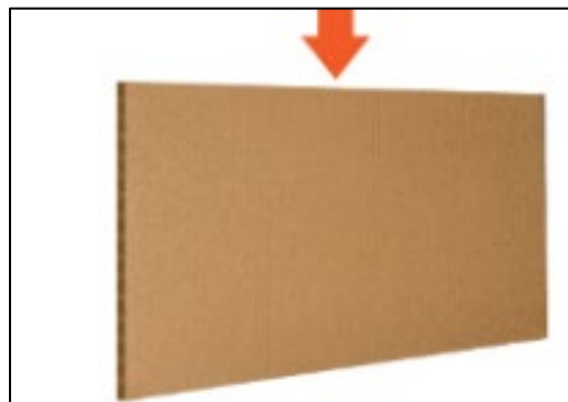
Figure 6. Edge crush testing of a corrugated board (Agrawal & Shetty, n.d.)
