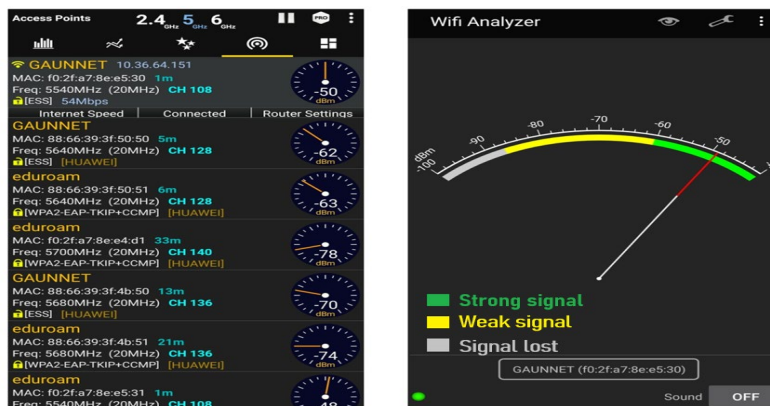
Figure 3. List of available internet access points in a distinguished area (left-side), alongside a signal strength meter (right-side).
