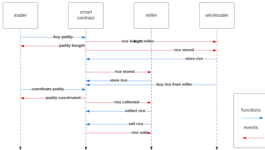
Figure 4. Sequence Diagram for Representing the Interaction Between Trader, Smart contract, Miller and Wholesaler.
