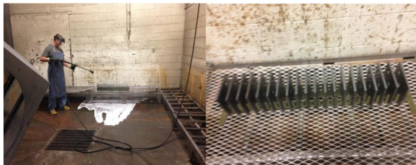
Figure 1. Cleaning samples in pressure wash area
