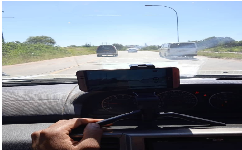
Figure 2. Pothole image capturing setup mounted on a Nissan X-Trail
