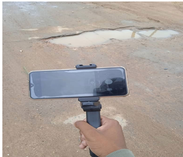
Figure 1. On-foot pothole image capturing setup.
