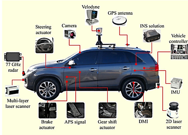
Figure 3. Sensor configuration diagram of the self-driving car used in the experiment
