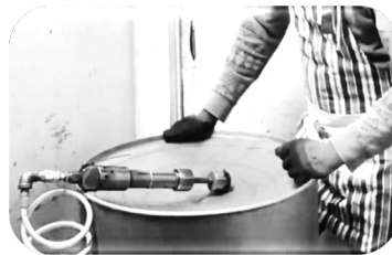
Figure 2. Incremental hammer forming tools for sinking pan.
