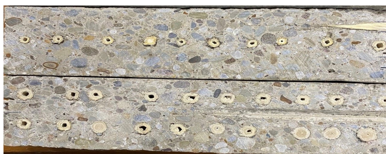
Figure 11. New Hemp stems reinforced concrete panel (0/90/0) t , cut in two perpendicular cross sections, yz and xz cross sections.
