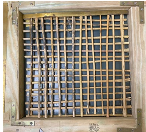
Figure 6. Preform for concrete pouring
