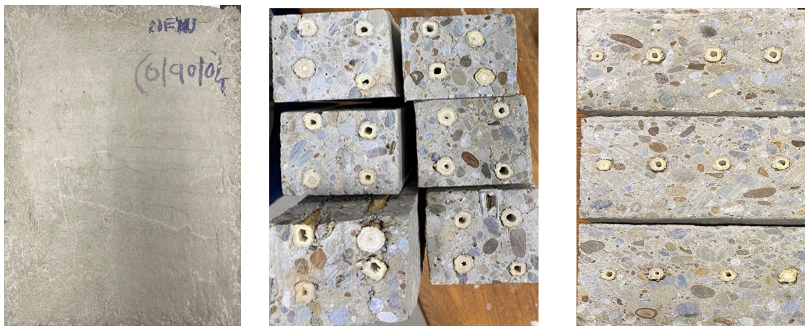
Figure 10. New Hemp stems reinforced concrete panel (0/90/0), and yz and xz cross sections.
