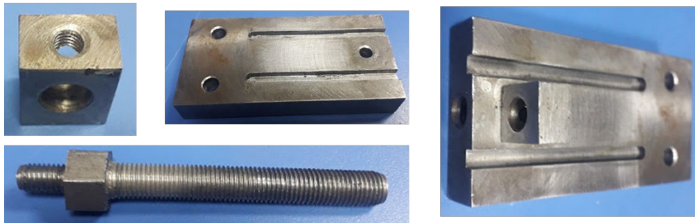
Figure 3. CAD of Locator Sliding Base (LSB) and the actual LSB along with its components.
