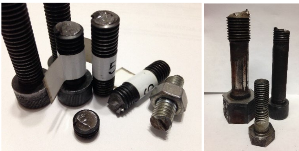
Figure 3. Failed bolts that have been collected for the study
