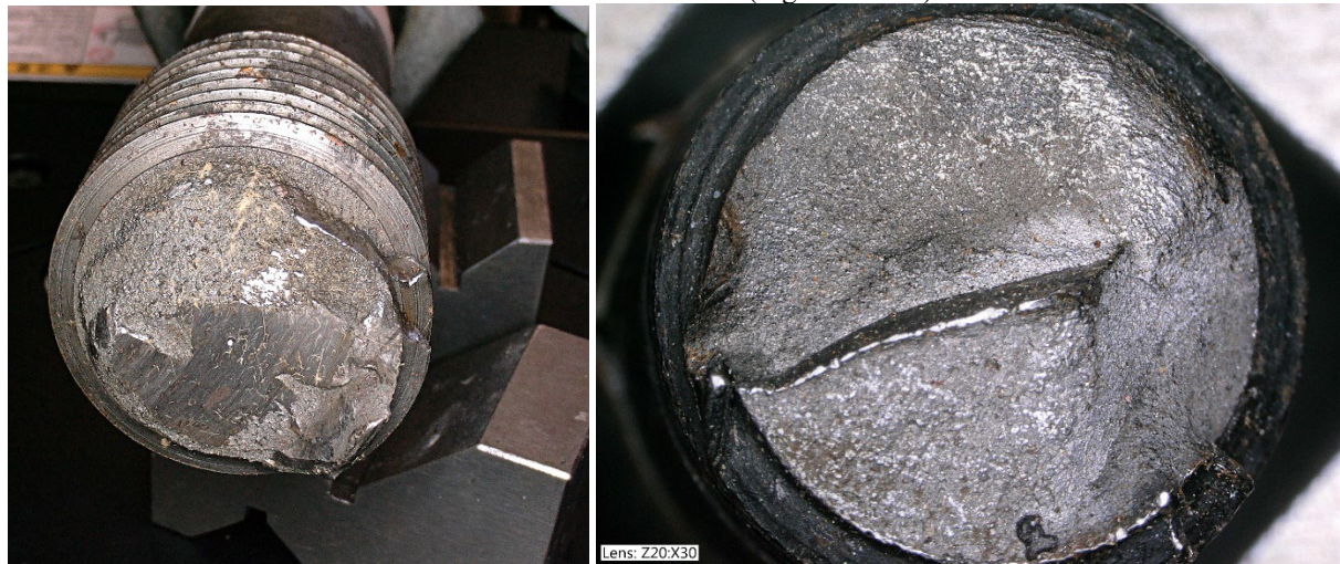
Figure 6. Failure due to a combination of shear and tensile overloads (Left), and due to high-cycle fatigue (Right).
