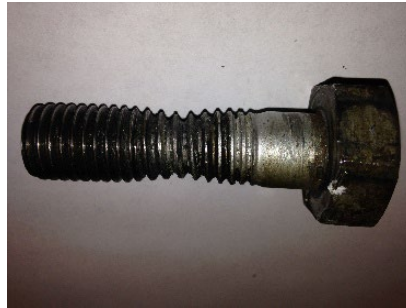
Figure 2. A bolt that failed from pure tensile overloads. The bolt underwent thinning and axial elongation, and was retrieved by the technicians before it fractured.
