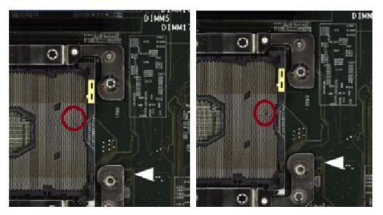
Figure 4. Case Study PCBA: "Before" (left) and "After" (right) AOI Images
