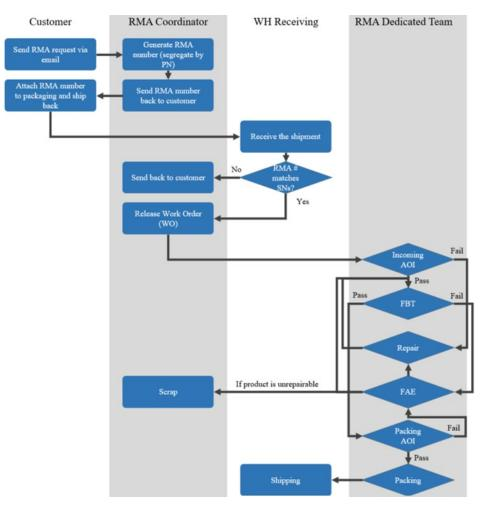
Figure 1. RMA Process for Electronic Manufacturing Company in USA
