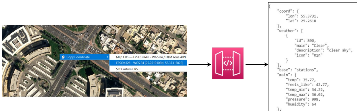
Figure 5: Example of OpenWeather API given location data for an area of interest. The API provides weather data such as temperature and humidity.
