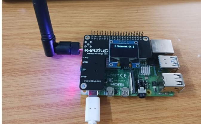
Figure 2. Gateway built using Raspberry Pi and LoRa hat.
