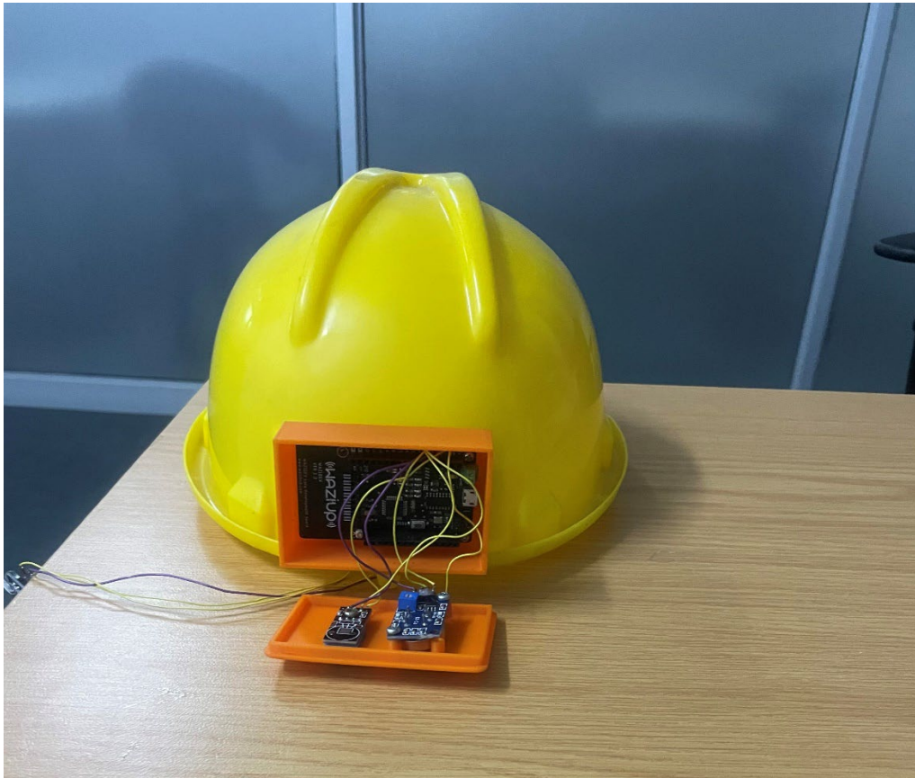
Figure 4. Smart Helmet showing WaziDev and the MQ2, DHT11 and MAX30105 sensors.
