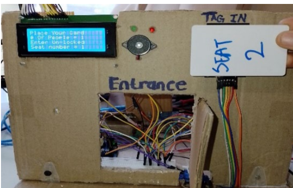
Figure 8a. Servo motor rotating +90 degrees to open the door when the RFID tag was tagged on the reader
