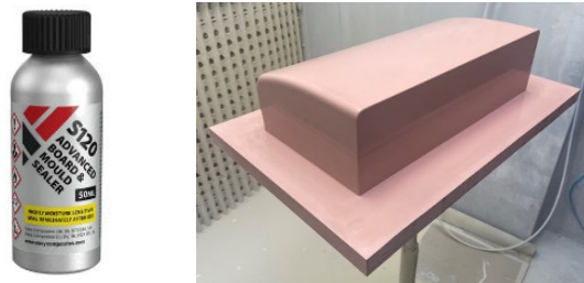
Figure 6. S120 board sealer (left) and master plug after finished surface preparation process.
