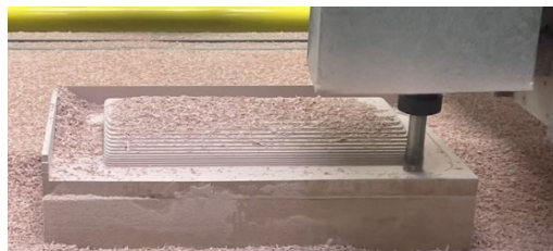
Figure 5. Master plug machining.
