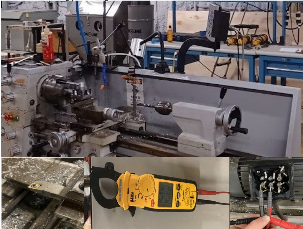
Figure 1: The machining setup with UEi DL 599 Wireless three-phase clamp meter and tool cutting angle for the experimentation
