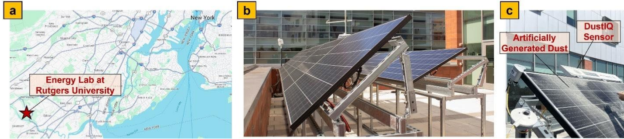
Figure 2. (a) Location of the Energy Lab at Rutgers University, New Brunswick; (b) Profile view of the PV system under study; (c) The DustIQ Sensor, mounted to the solar panel, showing artificially generated dust
