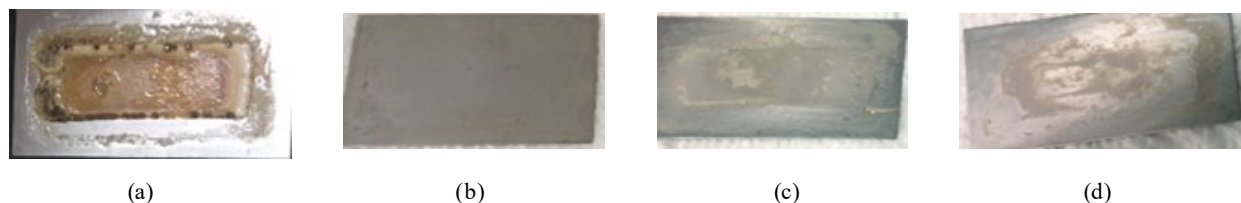
Figure 2. Coconut milk foulants (a) before cleaning and after cleaning by (b) NaOH and by a mixture of Celluclast® and Protease (Acalase) at (c) 50 rpm for 4 hr and (d) 55 rpm for 2 hr.
