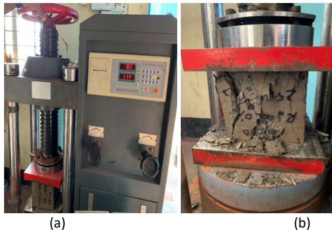
Figure 7. Compressive strength: (a) loading time on the cube, and (b) after applied maximum load.
