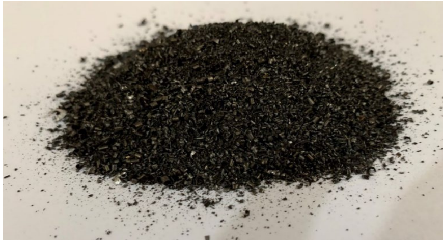
Figure 1. Recycled iron powder is used as fine aggregate in concrete.
