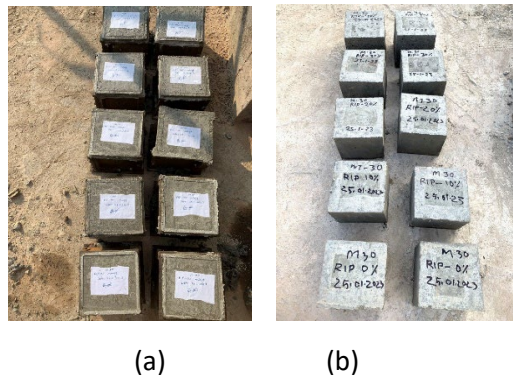
Figure 4. Test samples: (a) after compaction and (b) marked samples after roving from molds.
