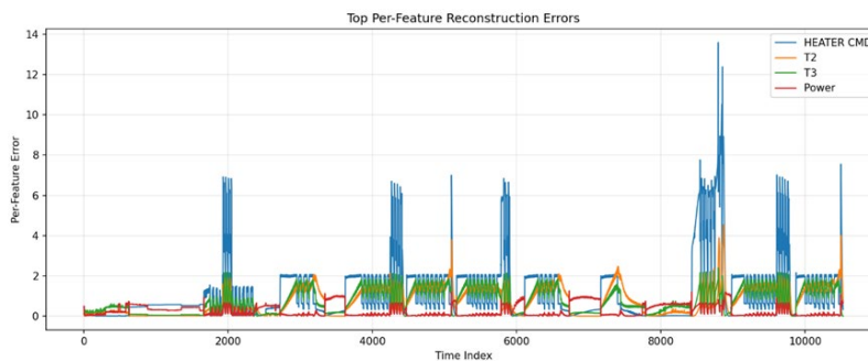
Figure 5. Feature-based reconstruction error distribution for faulty test data
