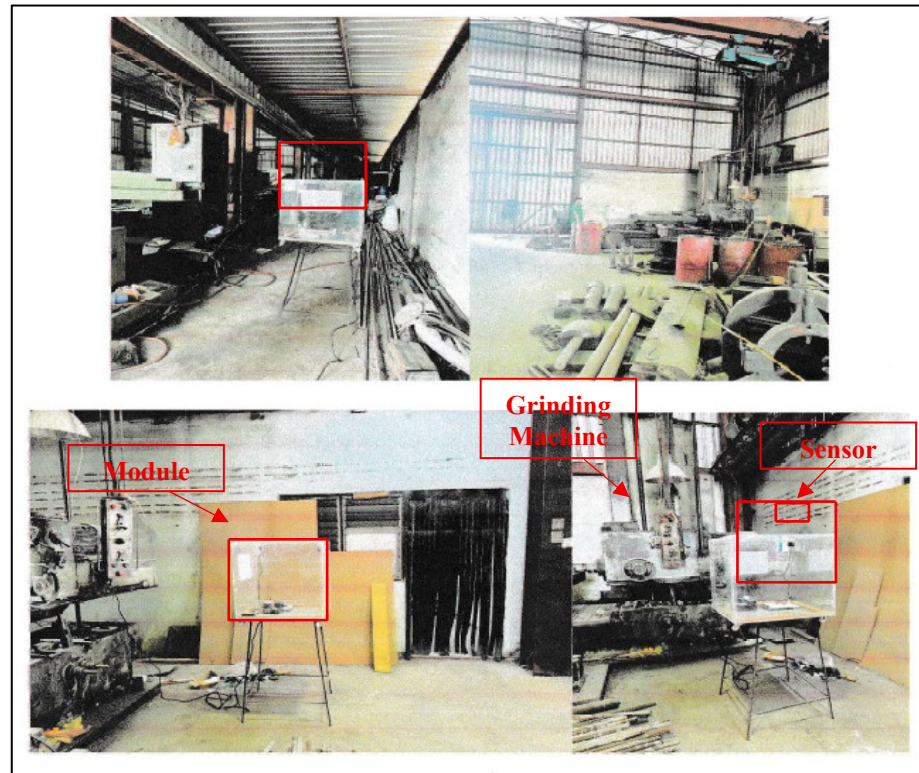
Figure 3. Field deployment of the IoT noise monitoring module within the grinding machine
