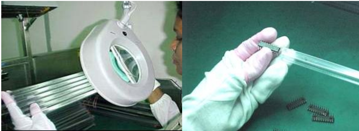
Figure 1: Use of luxor lamp and magnifier for IC Inspection and procedure of removing defective unit.
