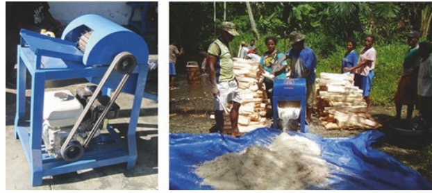
Figure 1. Overall structure of improved cylinder-type sago rasping machine.
