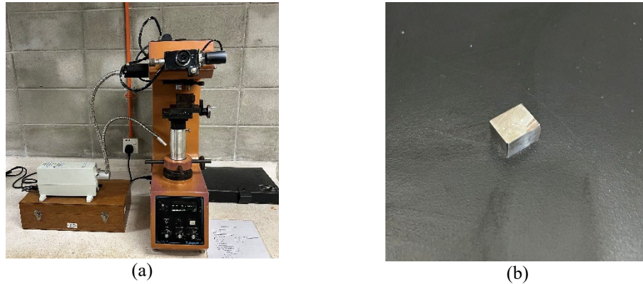
Figure 5. (a) Vickers Hardness Machine; (b) Specimen undergoes Vickers Hardness Test
