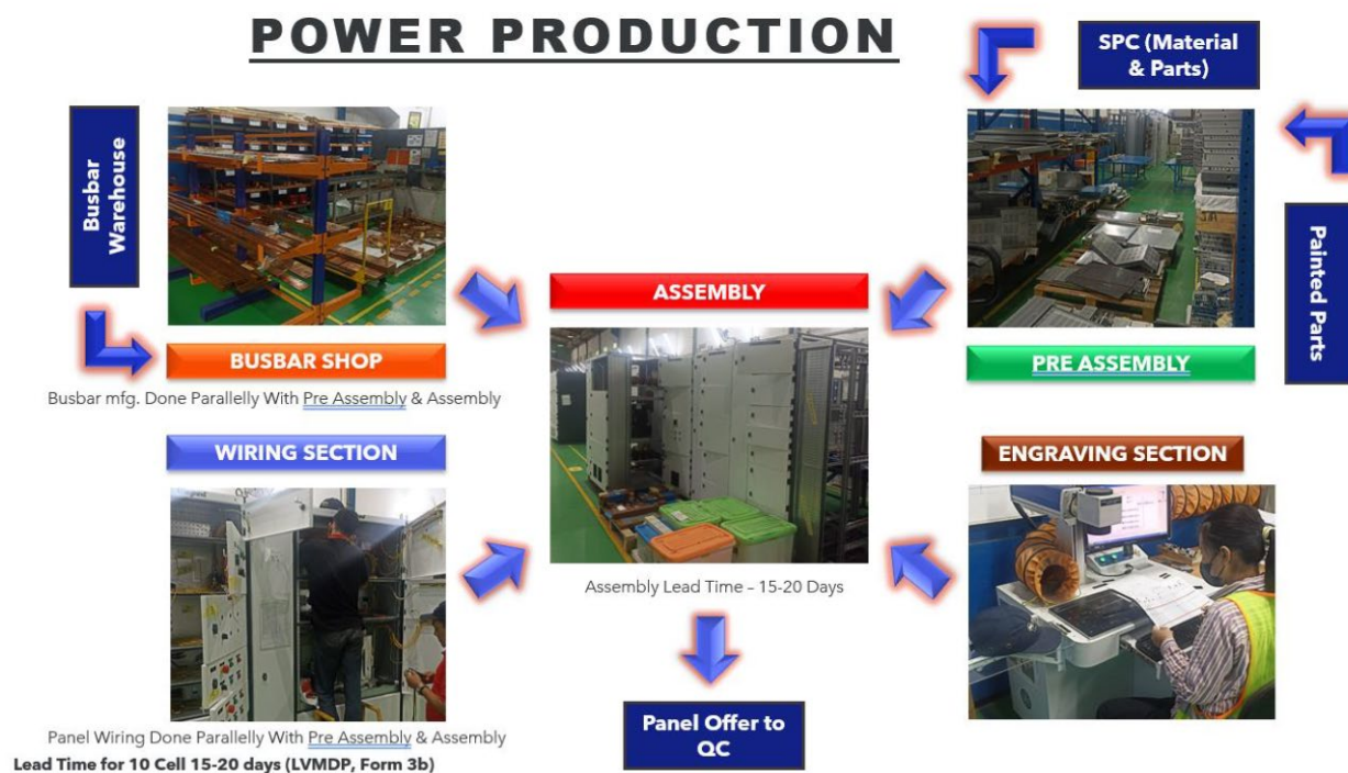
Figure 2. Electrical panel production process
