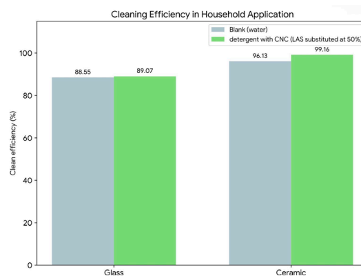
Figure 3. Comparative results of oil stain removal efficiency
