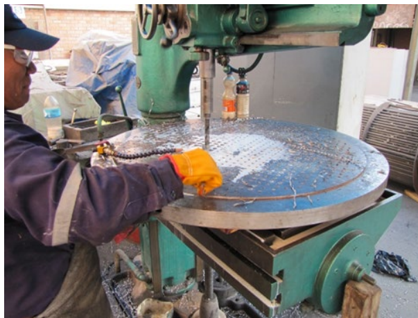
Figure 3. Drilling of a baffle
