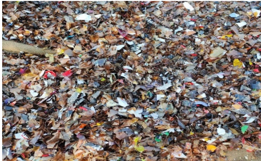
Figure 3. Low-Quality PET flakes with varied flake sizes, unsorted colors, and PVC contamination
