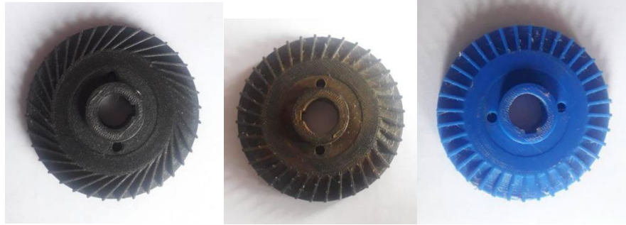
Figure 2. 3D Printed Impellers with 40°, 70° and 90° Blade Exit Angle
