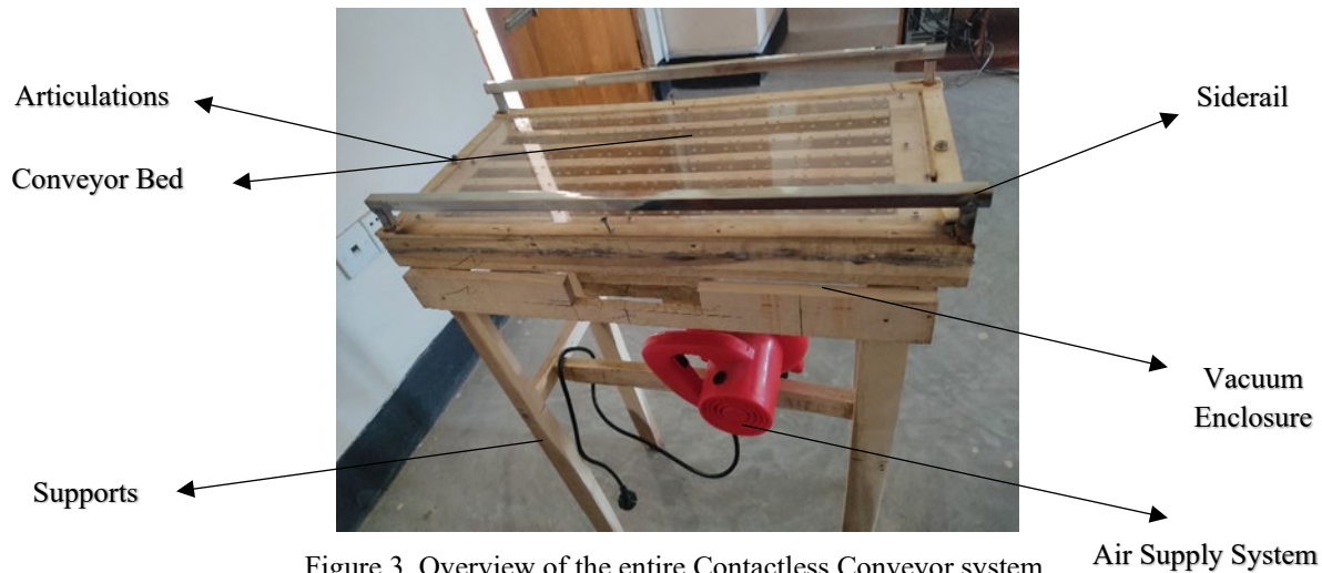
Figure 3. Overview of the entire Contactless Conveyor system.
