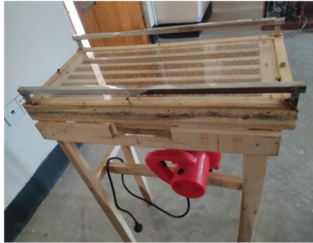
Figure 1. Experimental setup of an Air Conveyor
