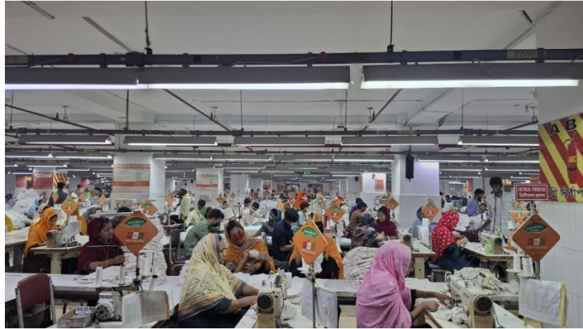
Figure 2. Sewing Line with Manual Material Handling System
