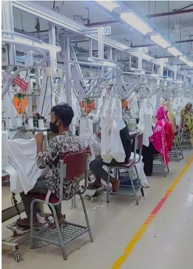
Figure 4. Sewing Line with Overhead Automated Material Handling System
