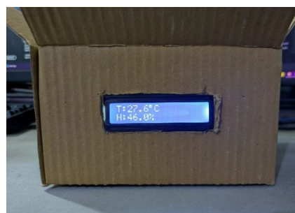
Figure 9. 16X2 I2C LCD for displaying real-time temperature and humidity.
