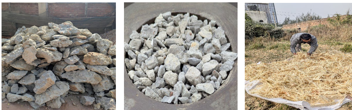
Figure 2. Waste materials used in this study (demolition waste, recycled aggregate, sugarcane husk)
