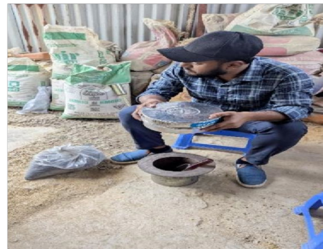
Figure 6. SHA sample preparation burning & sieving
