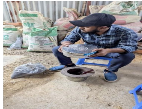
Figure 6. SHA sample preparation burning & sieving
