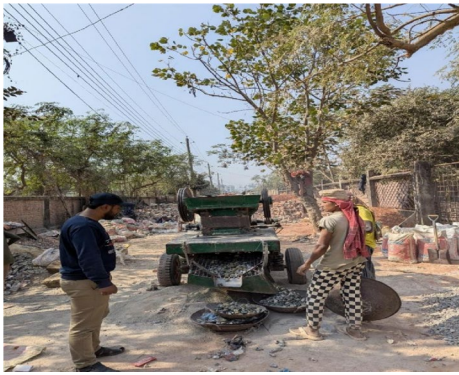
Figure 5. RA sample preparation crushing & sieving
