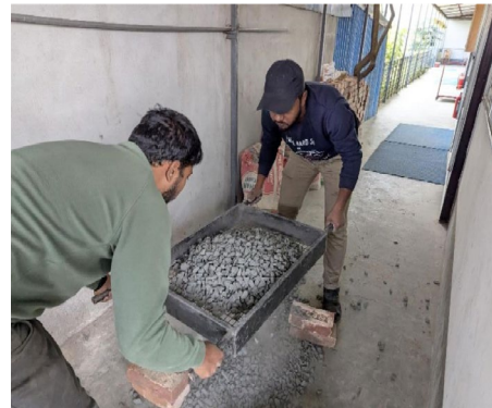
Figure 5. RA sample preparation crushing & sieving
