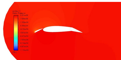
Figure 14. Static pressure contour of NACA 2415 airfoil at 15° plain flap deflection at critical AOA 19°
