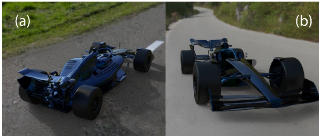
Figure 1. Comparative illustration of a Formula 1 rear wing, (a) DRS on and (b) DRS off.
