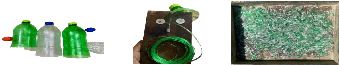
Figure 2 Left: Waste plastic bottles; Middle: Handmade cutting machine; Right: Drying process of cleaned plastic fibers.
