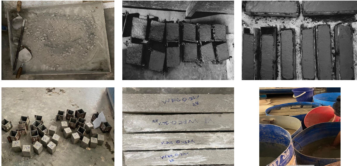
Figure 3 Fresh concrete mixing, cube and beam casting, demolding and curing process.
