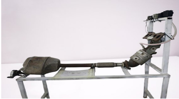
Figure 10. Photo of the exhaust system mounted on the frame.
