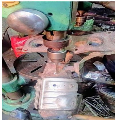
Figure 8. Photo of drilling between O 2 sensor and catalytic converter.
