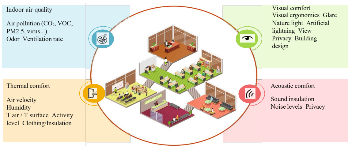
Figure 1. Overview of indoor environmental quality.
