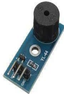
Figure 3. DC Buzzer a vibrational device
