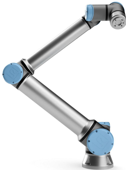
Figure 1: UR10 six-DOF industrial manipulator used in this study.
