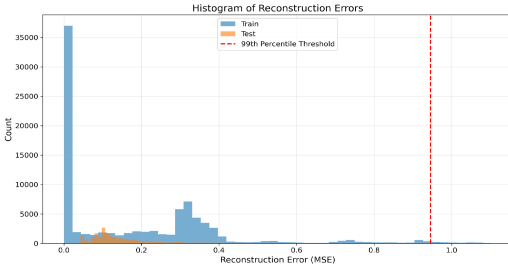
Figure 4. Distribution of reconstruction errors obtained from the LSTM autoencoder for training (normal) and test windows.
