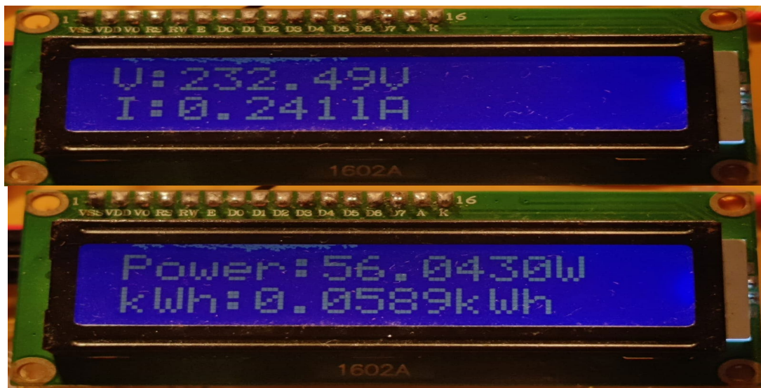
Figure 10: Value of Voltage, Current Power & Consumption for Double Load
