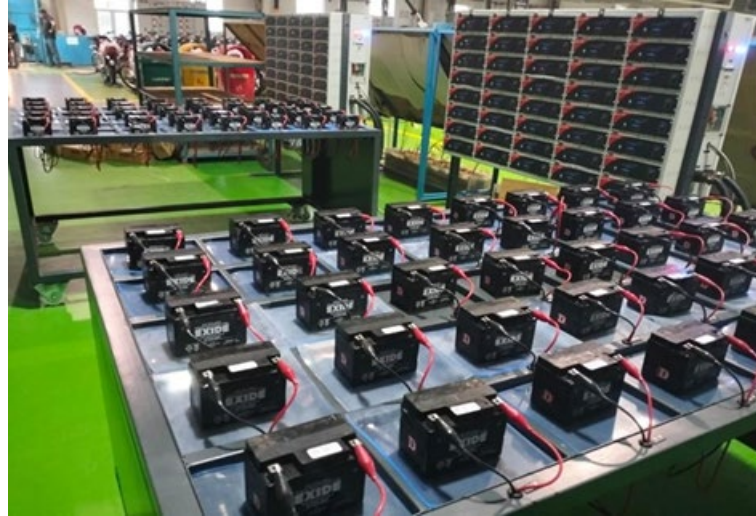
Figure 9. In-plant battery charging station with five units for enhanced battery maintenance and quality control.
