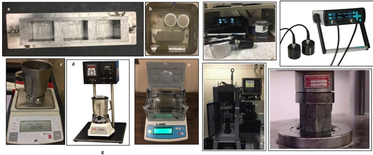
Figure 1. Experimental testing of the samples - curing of samples in temperature-controlled water baths, stress testing and acoustic testing
