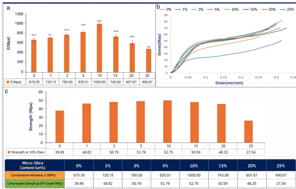
Figure 5. Mechanical properties of solid polypropylene/micro-silica composites: (a) compression modulus (E), (b) compressive stress–strain curves, and (c) compressive strength at 10% strain as a function of micro-silica content.
