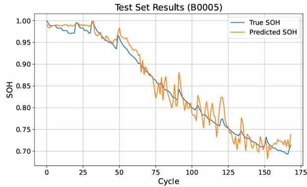
Figure 3. Basic PINN SOH prediction on Battery B0005. Predicted SOH closely follows the true degradation trend, with increased oscillations in later stages where nonlinear degradation effects become prominent.
